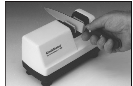
Stage 1. “Breaking-in” knife in Stage 1 will take 15 to 20 passes through each slot, alternating left and right slots. Subsequent resharpenings require fewer passes in Stage 1. Apply light to moderate downward pressure.
