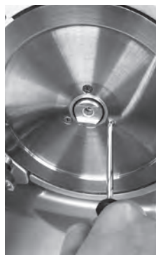
Figure 7c. Remove retaining screws.
