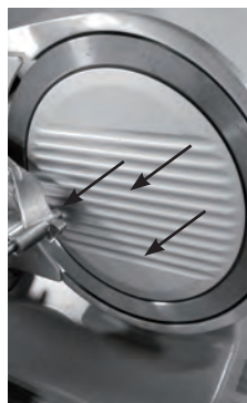
Figure 7b. Pull off blade guard.
