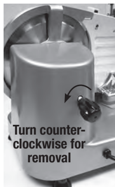
Figure 7a. Turn blade guard knob.
