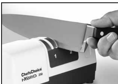
Figure 2. Inserting the blade in the right slot of Stage 1. Alternate pulls in left and right slots.
