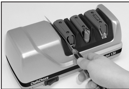
Figure 3. Stage 1. Inserting blade in slot between guide and flexible spring. Alternate individual pulls in right and left slots.
