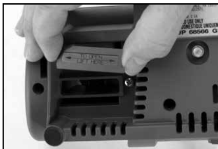
Figure 17. Removing cover under base to clean out metal dust (see Normal Maintenance section).
