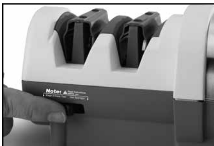
Figure 15. Use dressing tools sparingly.
