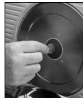
Figure 8. Turn the screw CLOCKWISE for blade removal.
