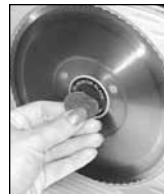
Figure 7. Turn the screw clockwise for blade removal.
