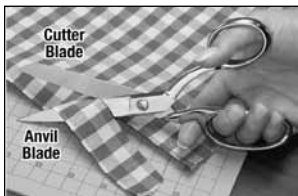
Figure 11: Typical position of the Cutter Blade and Anvil Blade on Right-handed Scissors.
