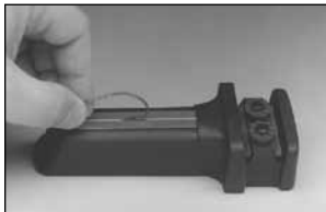
Figure 8: Using the fishhook sharpening pad: correct motion.
