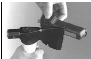
Figure 7: Sharpening an axe with the coarse pad.
