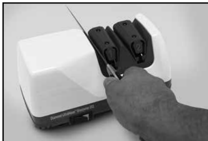
Figure 3. Stage 1. Inserting blade in slot between guide and elastomeric spring. Alternate individual pulls in left and right slots.
