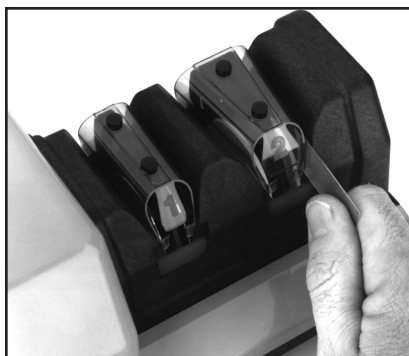
Figure 9. Dressing Stage 2 Honing Wheel.
