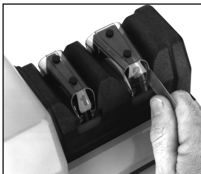
Figure 9. Dressing Stage 2 Honing Wheel.
