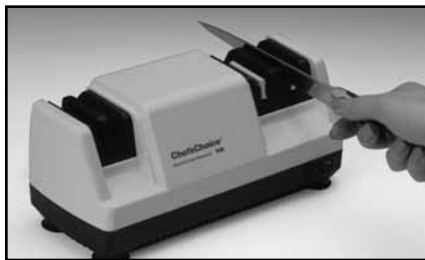
Stage 3— Eight (8) fast passes through each slot (left and right HONING slot). Alternate each pass.
