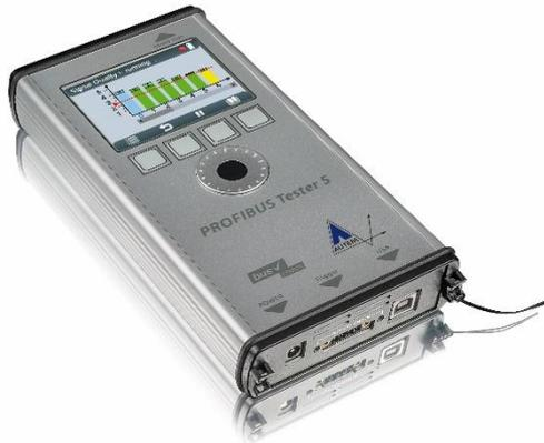
The **PROFIBUS-Tester V5** is a powerful diagnostic and troubleshooting tool for testing the cables, measuring the signals and analyzing the communication of PROFIBUS networks. Battery-powered and with an integrated graphical display it allows direct display of measurement results in stand-alone mode. In addition, the **PROFIBUS-Tester V5** supports the export of test results for advanced analysis.
