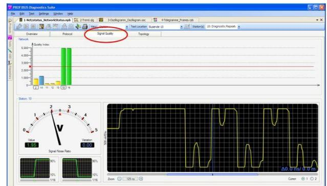
The **PROFIBUS-Tester V5** helps to save commissioning time. In addition, regular preventive tests ensure continuous reliable operation and increase plant availability. However, if a problem occurs, **PROFIBUS-Tester V5** will locate the reason quickly and reliably. Unplanned system downtimes will be minimized. The included software “PROFIBUS Diagnostics Suite” creates test reports of the current status of the PROFIBUS system in no time.
