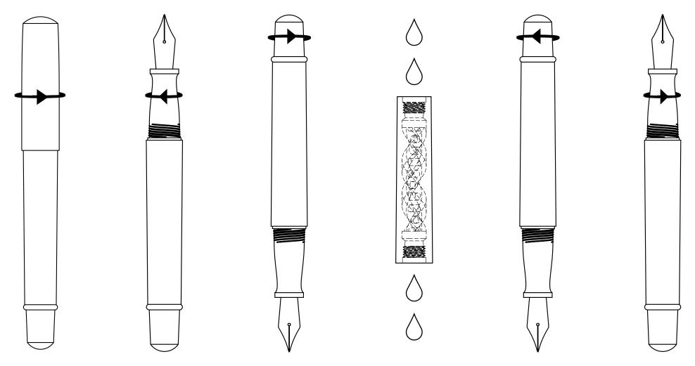
1. Unscrew the cap by twisting it counterclockwise.
