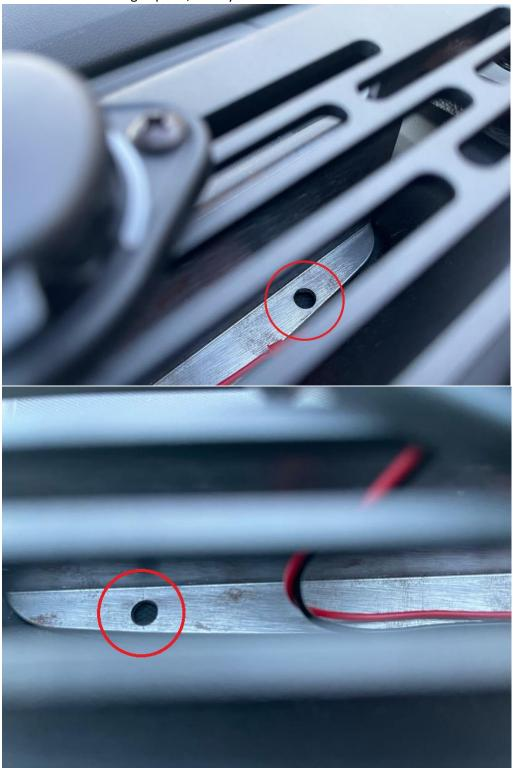
7. Remove the dash mount and drill your holes starting with he 1/8" as a pilot hole and finishing with the 1/4". If you purchased a charger, drill another hole towards the front or edge of the tray to pass the charger's wire.
