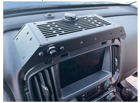
4. Loosely install the screws and slightly place the dash mount as high as it will go as shows below.
