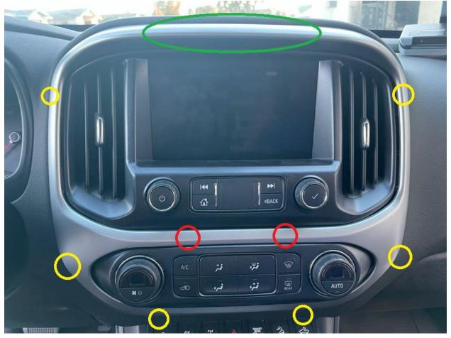
2. Remove the two screws circled in red.
