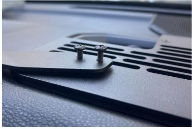
12. Once you snug the screws down, stick the brace onto the top of either A/C Vent.
