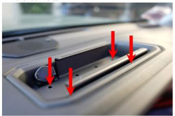
7. Using the provided 8/32 screws washers and nuts, bolt the base to the dash tray.
