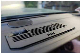
9. Screw the dash mount top to the base. If you will be installing the driver and passenger braces, do not install the pair of screws on either side.
