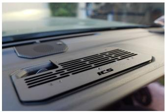
5. Using a thin Phillips screwdriver or pick, go through the slots and mark the 4 outer holes
