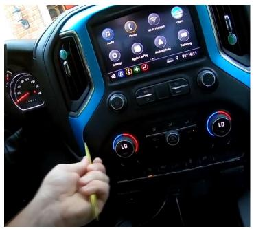
5. Now that you've gained access, remove the 4 or 6 (depending on your model) 7mm screws holding the radio/ac control assembly to the dash and lower it in place as shown in figure b.
