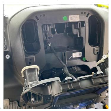
6. You will now see the tight space you have to work with as shown in figure c. Remove the top plate from the dash mount and drop in the lower dash mount plate onto the dash tray.
