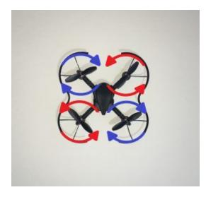
Blue propellers are marked A - Red propellers are marked B
