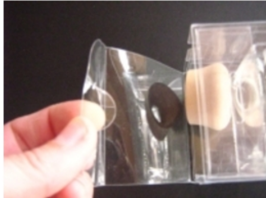
16. Close the base of the box first popping out the semi circle of plastic. This will fit into another slit in the long tube to securely close the lid
