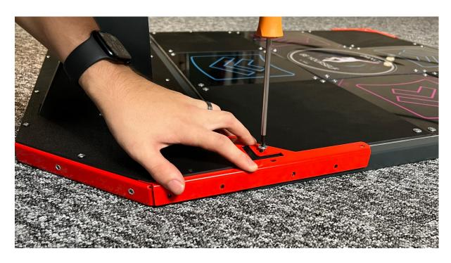
**STEP 4**: SCREW **9** SMALL M4 CREWS INTO THE MOUNTING HOLES
