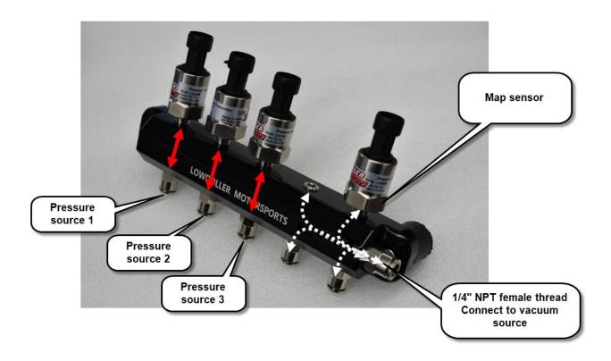
\*Starting on the right side\* The first (2) ports are common'd together with the end port being tied to the intake manifold. This will be used for the map sensor, fuel pressure regulator, blow off valve and anything else that needs a vacuum reference.
