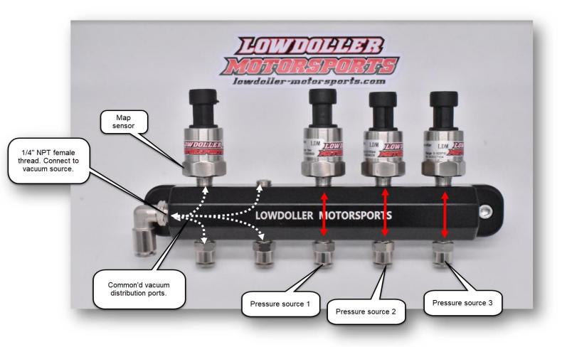
\*Starting on the left side\* The first (2) ports are common'd together with the end port being tied to the intake manifold. This will be used for the map sensor, fuel pressure regulator, blow off valve and anything else that needs a vacuum reference.
