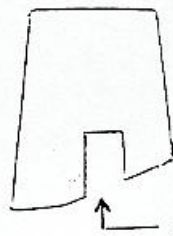
FIG. 5 Cut-Out Templet For Front Mounting Block
