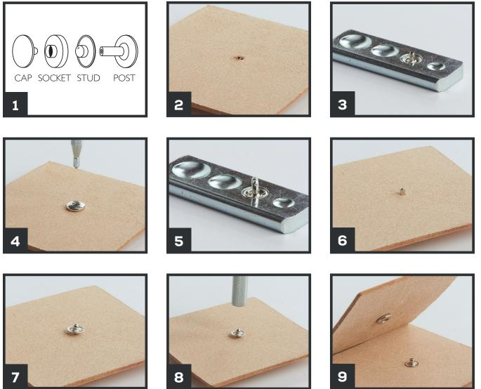
Place cap into corresponding size divet on the Anvil. Place pattern piece onto the cap. (Figures 2-3)
