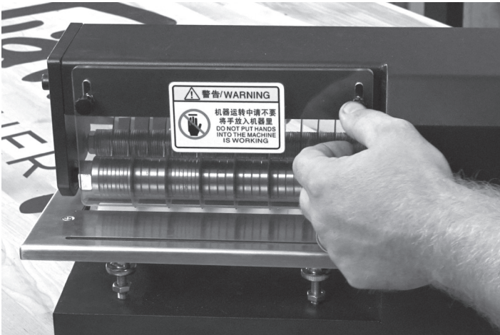
1. Unscrew the knobs holding the shield in place and remove it.
