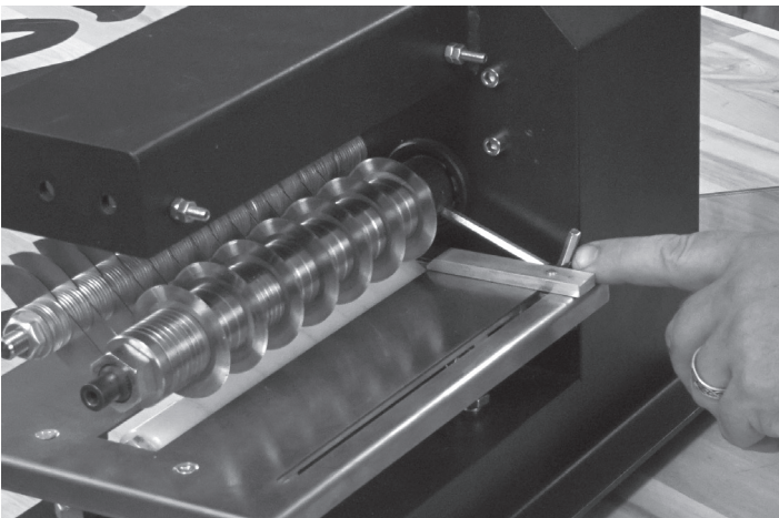
5. Insert an Allen key into the hole on the blade shaft to keep it from turning.
