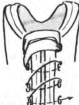
STEP 3. Continue lacing over and over, until you reach last hole.
