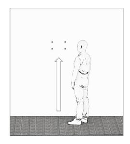
1. To determine the ideal height for your bicycle wall mount, use a marking pen to measure and mark a comfortable position based on your height and reach. Before drilling holes into the wall, make sure to check that the marks are level.
