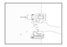
2. To securely install the bike mount, use a hand drill to drill Ø12mm holes where the M6 roll bolts will go. Once the holes are drilled, use a 10mm spanner or socket tool to fasten the roll bolts, which will cause the bolts to expand inside the wall and secure the mount in place. After this step, turn the M6 bolts counter-clockwise to loosen them, leaving the stud inside the wall.
