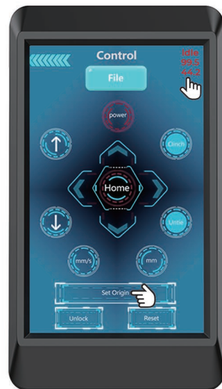
5. Adjust the coordinates of the upper right corner to be the same as the coordinates of the upper right corner of the machine. Finally click "Set Origin"
