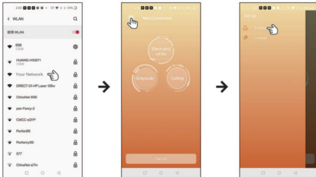
Connect to your network, open the App, click the gear in the upper left corner, click "Machine Settings", and enter the IP address in the offline interface
