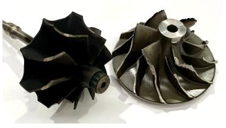
inevitable as the turbine and compressor wheels come into contact with their respective housings.
