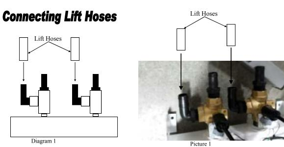
The lift hoses running from the lift tanks should be hooked up to the elbow fittings as shown in Diagram 1. Exhaust hoses can be added to the straight fittings to direct water away from the boat.
