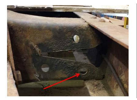
Shown is the rear passenger side of the cross member. To utilize this design the emergency brake cable will need to be removed from the large hole.
