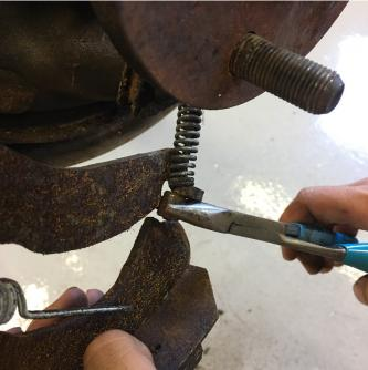
Remove the additional retaining springs from the brake shoes. Disconnect the parking brake cable from the brake shoe, then remove and discard the brake shoes and hardware.
