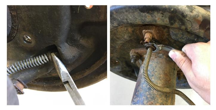
The cable can then be removed from the backing plate by depressing its perimeter springs. Remove the brake line from the wheel cylinder using a line wrench if possible.
