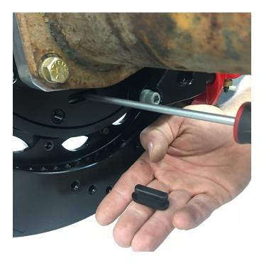
Adjust the parking brake shoes outward using a drum shoe adjustment tool (available at your local parts store) or a flat head screwdriver. You'll do this by spinning the rotor slowly until a slight drag is felt against the hat/drum. Remove the lug nuts that were holding the hat/rotor in place.
