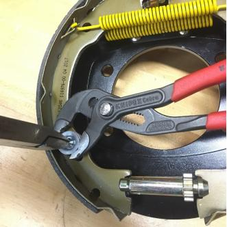
You will need to disassemble the parking brake assembly to install a new cable bracket. (This can be purchased separately as PN AFRC-B3300) Start by removing the retention springs as shown.
