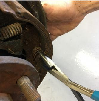
This installation refers to the passenger side of the axle. All steps are to be repeated on the driver side in kind. Start by removing the factory drum. It may be necessary use a lubricant around the axle register to do this. Once the drum is removed, remove the brake shoe retaining springs (2 places) as shown.
