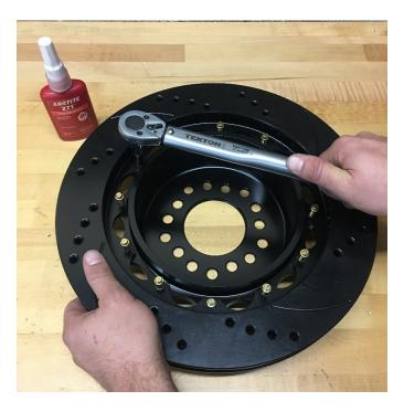
Arrange the rotor and hat in the position shown ensuring the arrow noting rotation direction is correct for its position on the vehicle. Start the first few threads of all 12 of the ¼-20 x .75 12-point bolts. Using an alternating sequence, apply red Loctite® 271 to the threads, and torque to 155 in-lbs. (Safety-wiring is not required for these bolts. If safety-wiring is desired/required for your application, then Wilwood PN 230-4572 can be used as an added measure of security.)
