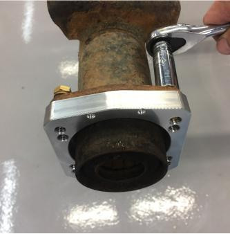
Make sure the surface of the axle flange is clean and deburred before installing the spacer. Install the machined spacer as shown using the hardware provided. The dimples will be mounted **UP** and **OUT** when installed properly.
