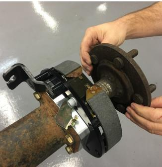
The parking brake assembly can now be installed onto the axle with the supplied hardware. The axle shaft can now be reinstalled per OEM recommendations.
