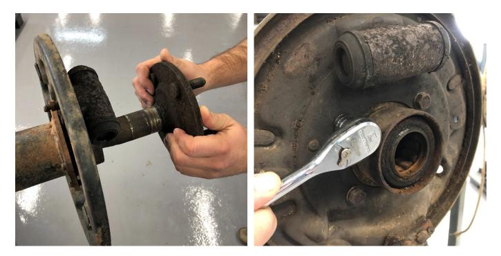
The axles will need to be removed from the housing by draining the fluid, then removing the differential cover and C-clip retainers. The 4 bolts retaining the drum backing plate to the axle can now be removed and discarded.
