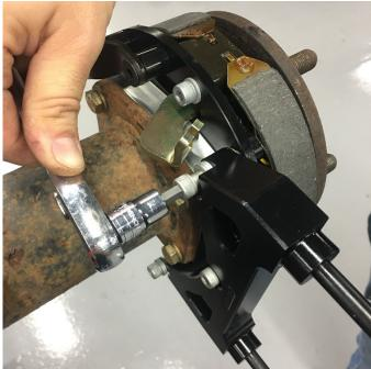
The socket head screw and washers should be assembled as shown above starting with the screw, 3 washers, the bracket, 1.625x.313x.015 shim washer, then the bracket spacer. You'll do this in 3 places. You can now bolt the caliper bracket to the emergency brake assembly and snug the bolts down. (You will not use threadlocker at this time) **NOTE:**The end of the screw should not exceed the insert and interfere with the brake shoe.
