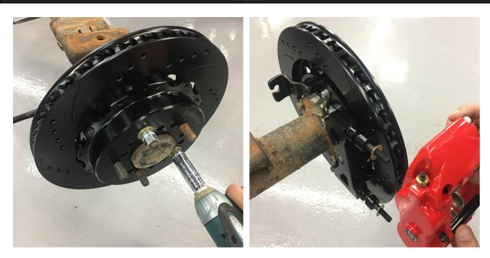
The rotor can now be installed using 2 lug nuts to temporarily secure it. Lubricate the caliper mounting studs with lightweight oil. Initially place one .875x.375x.035 shim on each stud of the bracket. Mount the caliper using lock nuts and washers and ensure that it fully seats on the bracket and does not contact the rotor.
