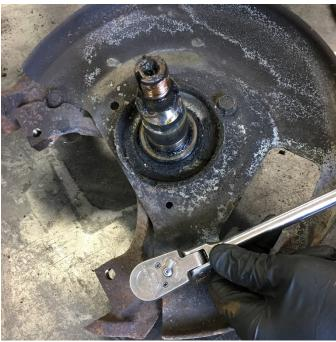
Remove the rotor to access the 3 dust cover bolts underneath. Remove the dust cover, which will not be reused.
