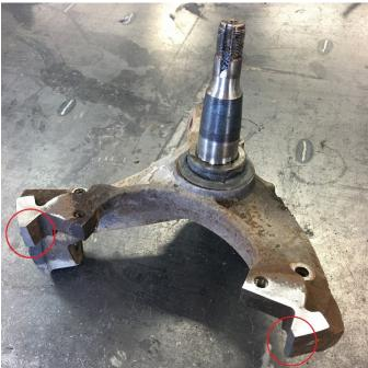
Trim the spindle ears as shown. A reciprocating saw, bandsaw, or cut-off wheel can be used. The sharp tips left over can be sanded flat as shown in Step 8 to avoid contact with the new caliper.
