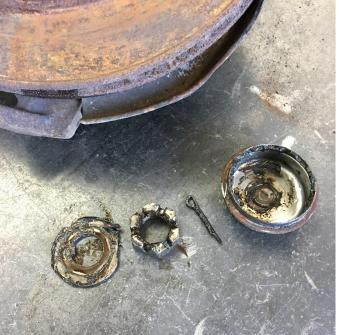
Remove the factory dust cover, then the cotter pin, castle nut, and washer. The castle nut and washer should be saved.
