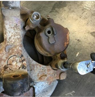
This installation refers to the passenger side spindle. All steps are to be repeated on the driver side in kind. For instruction purposes, the spindle has been removed. It is not necessary to remove spindle to install new brakes. Start by removing the factory brake line and factory brake caliper. These items will no longer be used
