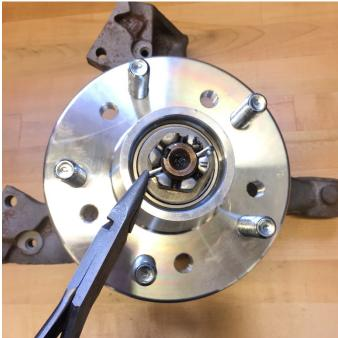
Pack the large inner bearing cone (A5) with high temperature disc brake bearing grease (available from your local auto parts store) and install into the back side of the hub. The inner seal can then me pressed in or lightly tapped in with a hammer by circling the perimeter. Install the hub onto the spindle, then pack the outer bearing (A3) with grease and install under the factory washer, castle nut, and supplied cotter pin.
