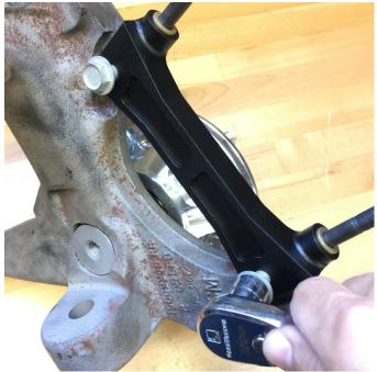
Install the dust cap by tapping lightly around the perimeter. The radial brackets can temporarily be installed at this time using the supplied flange bolts and two .750x.438x.035 shim washers between the bracket and the spindle. Any corners or burs on the spindle should be removed so that the brackets sit flat against the machined surface. It is not necessary to torque them at this time.
