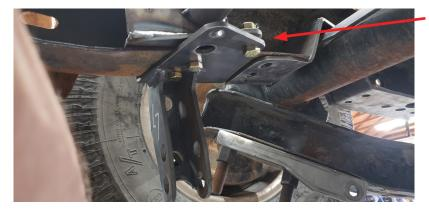
Shim plate for the frame bracket goes here.
