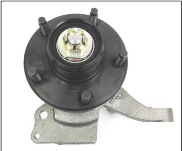
2. Apply a small amount of grease onto the Hub Seal and Slide the Hub Assembly onto the spindle. The Bearings are prepacked with synthetic grease. Do not add more grease. Tighten the spindle nut to 5-10 ft·lbs
