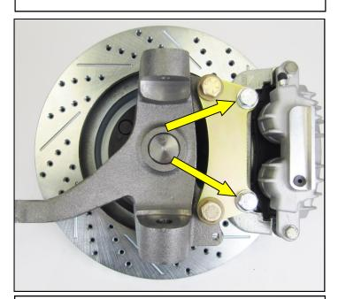
7. With the Brake Pads installed, slide the Caliper onto the Rotor as shown. Slide the Spacers between the Caliper and the Bracket and secure the assembly using the two 14mm Hex Head Bolts and washers. Torque the Bolts to 105 ft.lbs.
