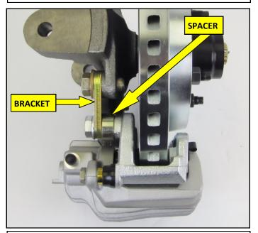
8. TOP View of assembly illustrating the relationship between the Caliper, Spacer, and Bracket.
