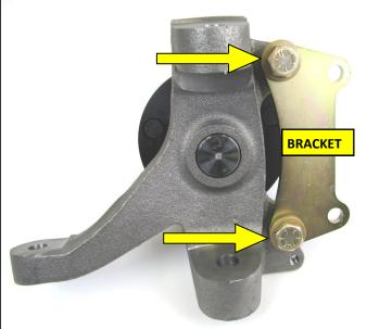
4. Install the Bracket onto the Inboard side of the Spindle using the 5/8"-18 Hex Head Bolts and Washers. Torque the Bolts to 240 ft.lbs.
