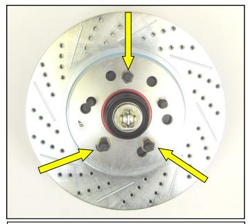
6. Mount the correct side Rotor onto the Hub Assembly and temporarily secure it using 3 nuts and washers.
