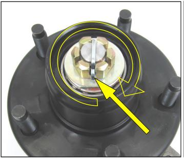
3. Rotate the Hub to seat the Bearings. Loosen and re-tighten the Nut while spinning the Hub several times. Tighten the Nut again, to remove all play, approximately 1/16th turn to give a small amount of pre-load. Install the Cotter pin as shown.
