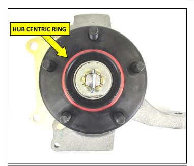
5. Slide the Hub Centric Ring onto the Hub with the beveled edge against the face of the Hub.
