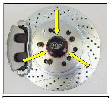
9. Lubricate the Dust Cap O Ring using the supplied Grease and install it onto the groove on the back side of the Cap. Place a shop towel over the face of the Cap to protect the surface and gently tap it into the Hub using a dead blow hammer or rubber mallet.
