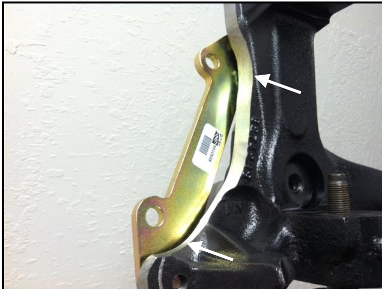
Figure 5: Grind away material so that the spindle does not interfere with caliper bolts
