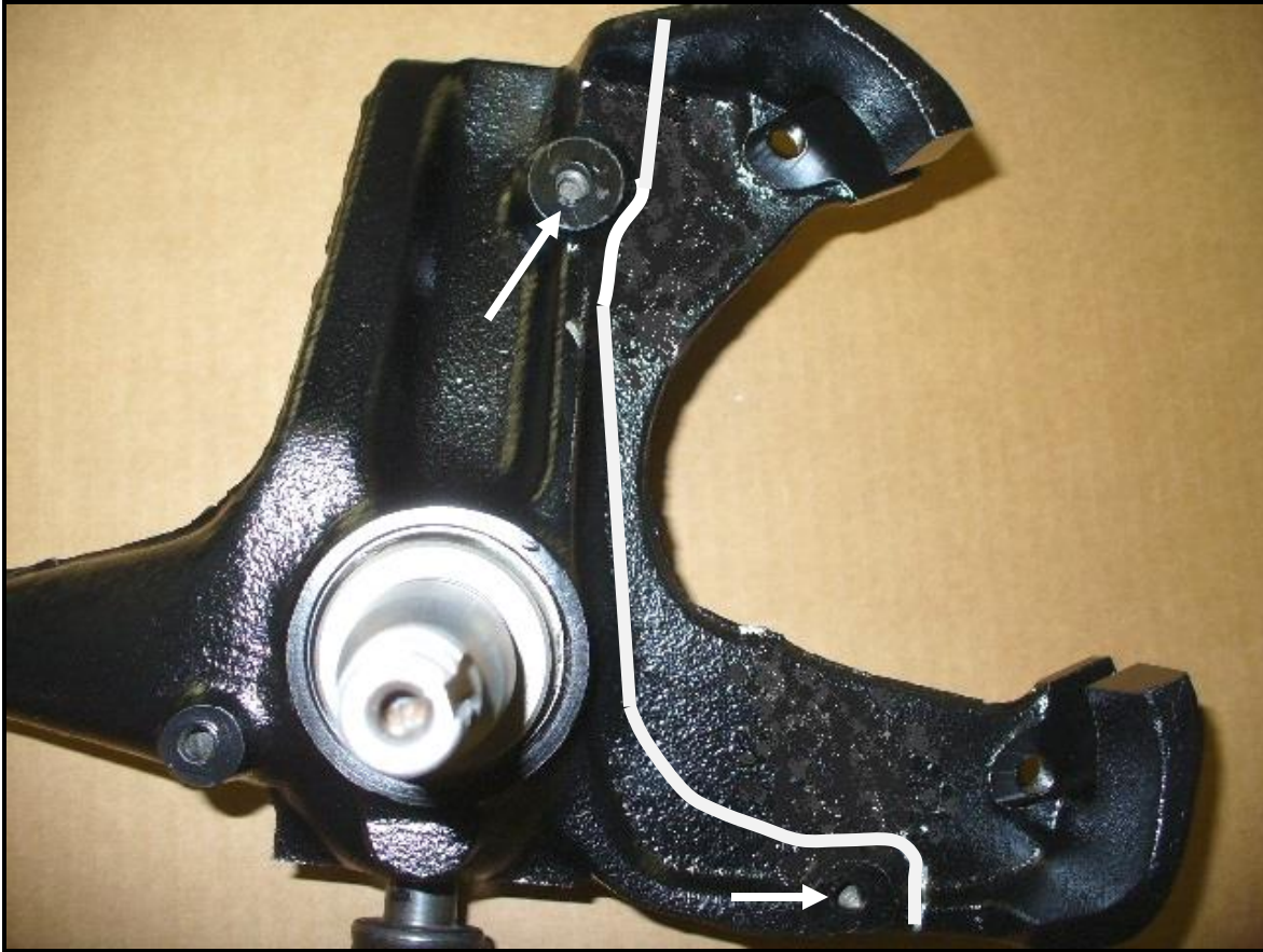
Figure 3: Arrows indicate debris shield mounting points that require drilling and tapping.
