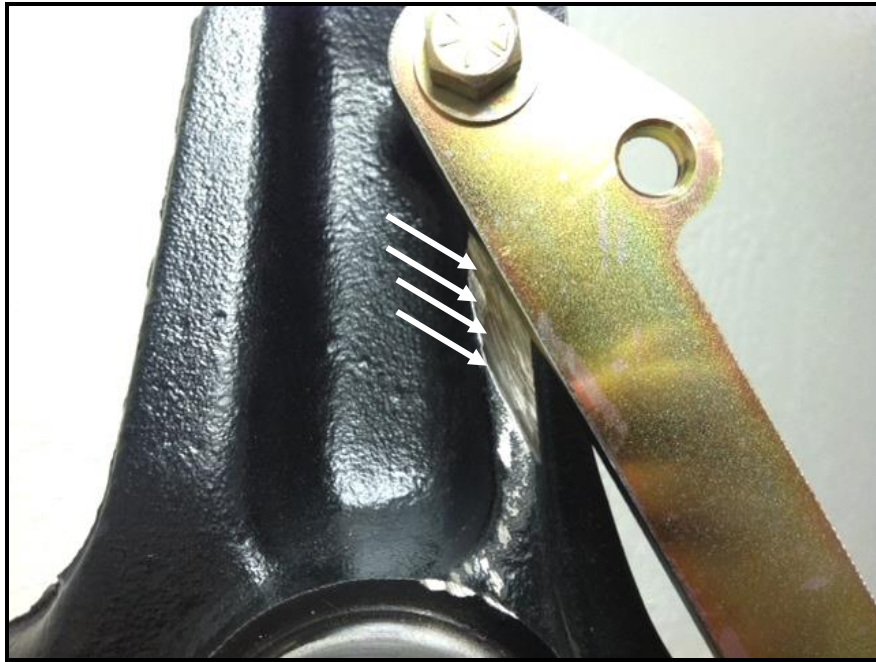
Figure 6: Material has been removed to allow for the bracket to seat properly
