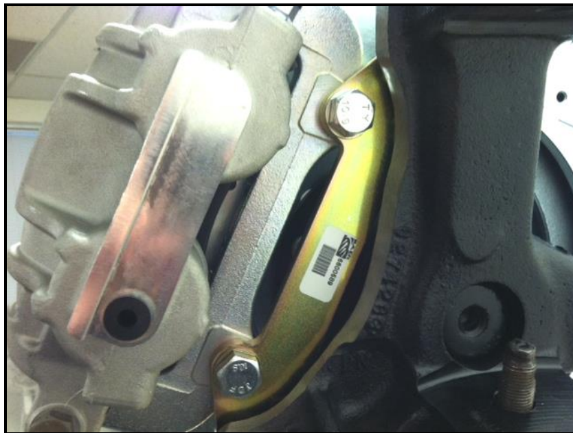
Figure 8: Caliper and bleeder clearance
