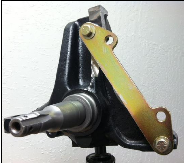
Figure 4: Caliper bracket installed onto spindle
