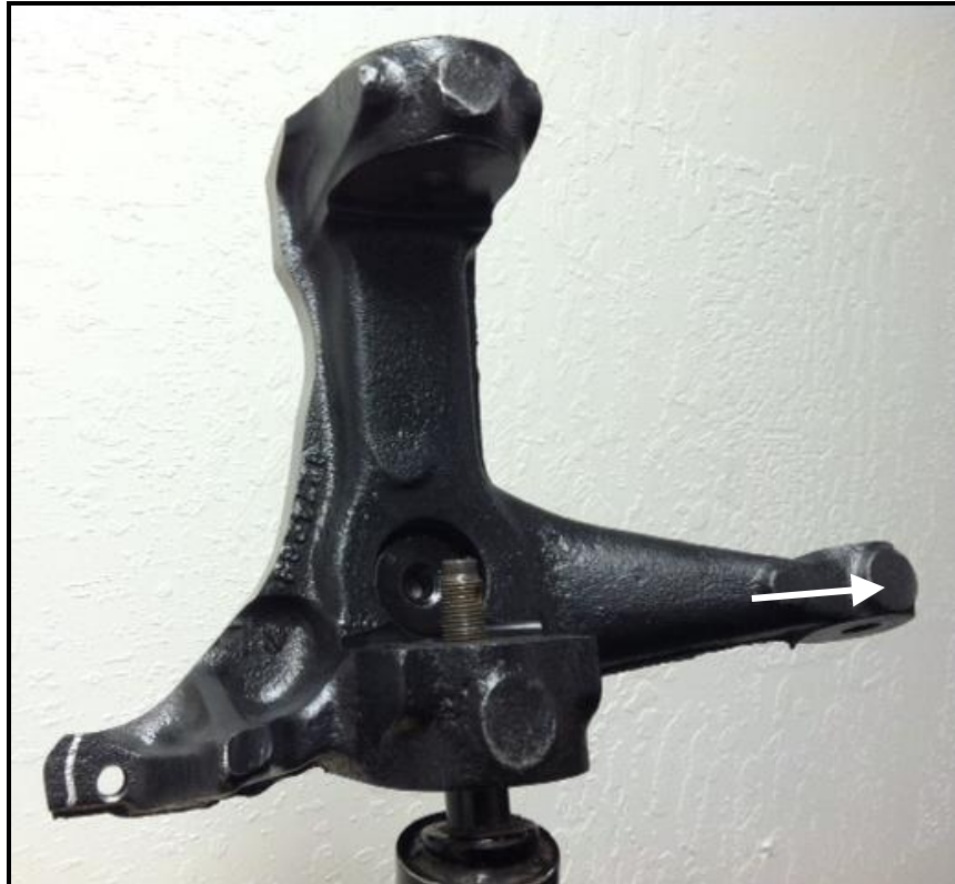
Figure 1: Strike steering arm boss at spot indicated by arrow
