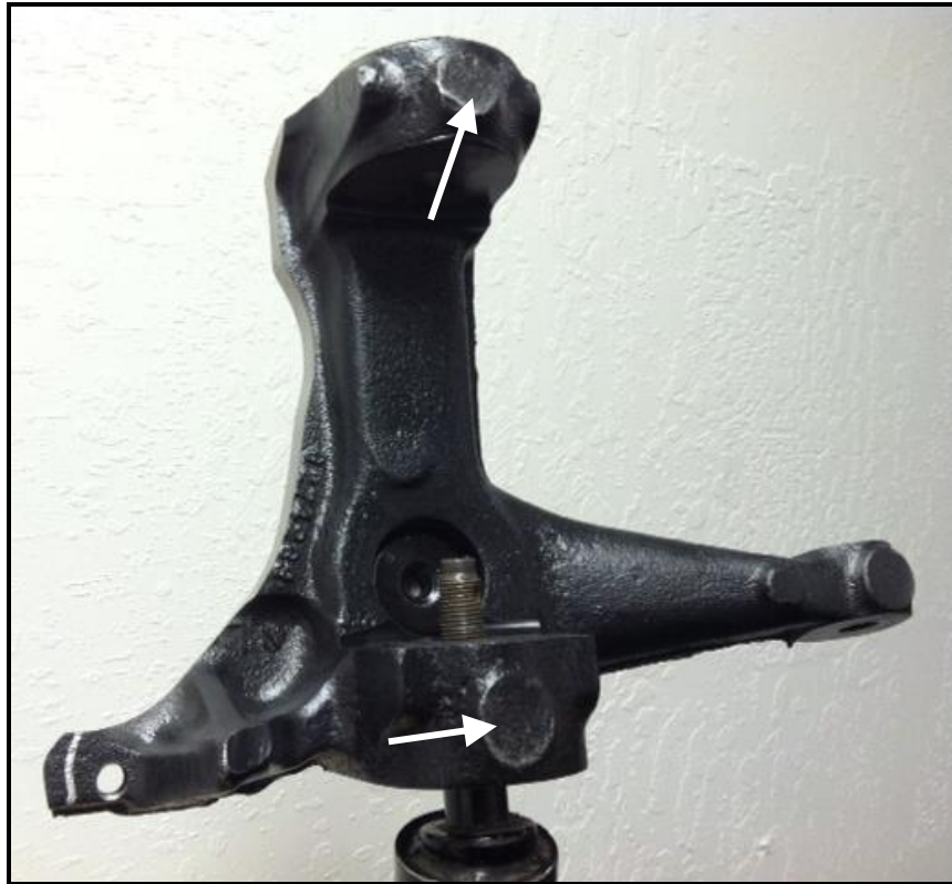
Figure 2: Strike tie rod end bosses with large hammer. Arrows show locations
