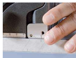
3. Align the Zeta P2 with the marking
