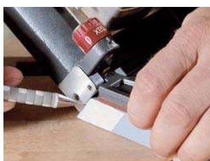
1. Cut and mark the center of the cut
