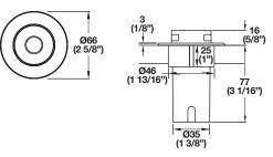
Requires a 47 mm hole in work surface for mounting
