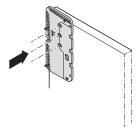
The positioning pins are pre-mounted in accordance with the selected door overlay dimension; then the drilling jig is positioned in both top corners of the door panel (reference mark "F")
