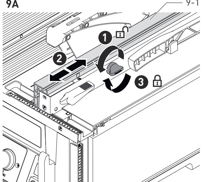
**i** Rotate [9B] the stop rail [9-1] for angled cuts or very small workpieces. The lower side then points towards the saw blade.
