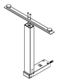
ASSEMBLE THE FOOT TO THE COLUMN
