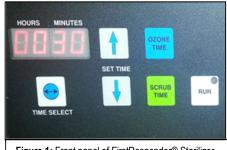
Figure 1: Front panel of FirstResponder® Sterilizer
