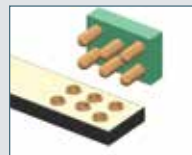
PRESS-FIT BUSHINGS WITH CROWN BAND INSERTS
