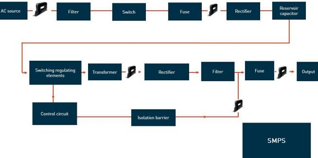
SMPS (Switched Mode Power Supplies) is a complex application with lots of components that it can be interesting to survey. The goal is to survey the main and strategic components in order to install the RFCS current sensors into your grid. First of all, we begin with AC source with 3 phases and 1 neutral and directly, we will filter this signal in order to eliminate the high frequency disturbance received or sent to AC source for example.
