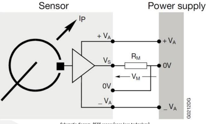
Schematic diagram: RFCS sensor (open loop technology)
