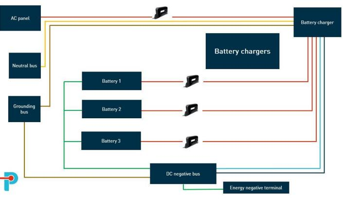
Each battery charger can be an opportunity to use our RFCS current sensors on each battery (3 RFCS in total) and upstream the battery charger linked to the AC panel (3 more RFCS sensors). Each battery (1 phase/DC) is linked to the battery charger. Each battery is connected to DC negative bus in order to close the electrical circuit.
