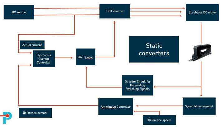
Each brushless DC motor are linked to RFCS current sensors (Hall sensor) on each phase of the motor. The RFCS will measure instantaneously on each phase the current. On the one hand, this value will serve for controlling the speed measurement as well give the value to the decoder circuit for generating switching signals.
