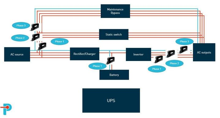
Internal design of a multi-mode UPS.
