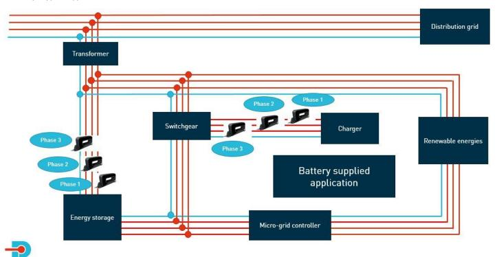
Each renewable energies (windmill, solar...) is either connected to the micro grid controller or the transformer. The energy storage is an assembly of a battery (in series and/or parallel), consequently, it can be mandatory for your application to install on each phase one RFCS sensor due to the fact you can have a variation of a significant current on the network.
