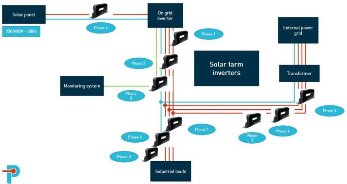
The electrical grid starts from the solar banel in DC current and bass over the inverter that converts DC current to AC currents. Then, everything is connected to the industrial load that refers to the bower consumption of the device(s) that are being used in the system. Understanding your loads is critical to maintaining a well-functioning power system.
