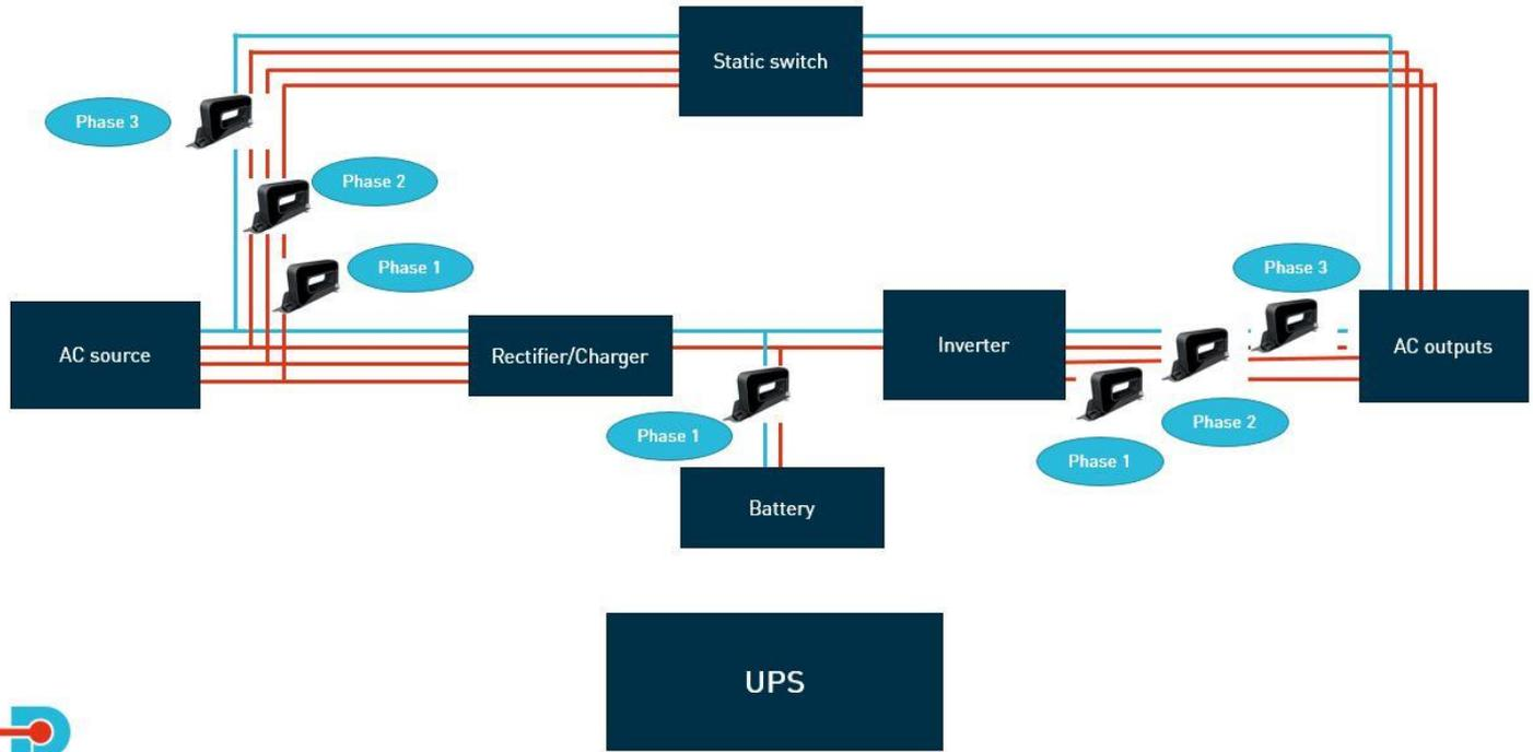
Internal design of a double-conversion UPS.
