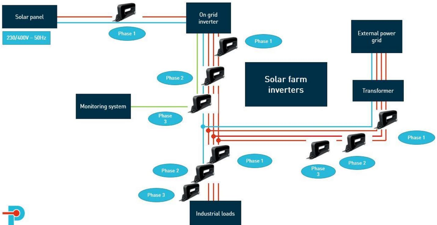
The electrical grid starts from the solar panel in DC current and pass over the inverter that converts DC current to AC currents. Then, everything is connected to the industrial load that refers to the power consumption of the device(s) that are being used in the system. Understanding your loads is critical to maintaining a well-functioning power system.
