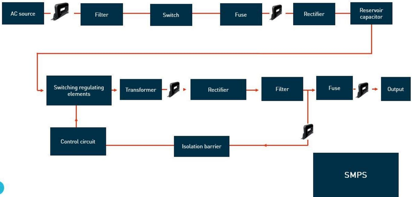
SMPS (Switched Mode Power Supplies) is a complex application with lots of components that it can be interesting to survey. The goal is to survey the main and strategic components in order to install the RFCS current sensors into your grid. First of all, we begin with AC source with 3 phases and 1 neutral and directly, we will filter this signal in order to eliminate the high frequency disturbance received or sent to AC source for example.
