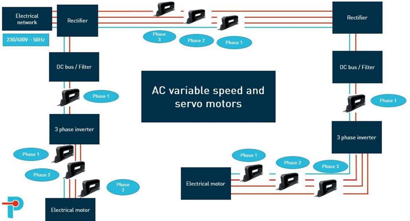
Each electrical motors are needed for running fans or compressors for example and are directly connected to 3-phase inverter. A three-phase inverter is an electronic device that converts direct current (DC) power into three-phase alternating current (AC) power. It is a crucial component in many electrical systems where a three-phase power supply is required.
