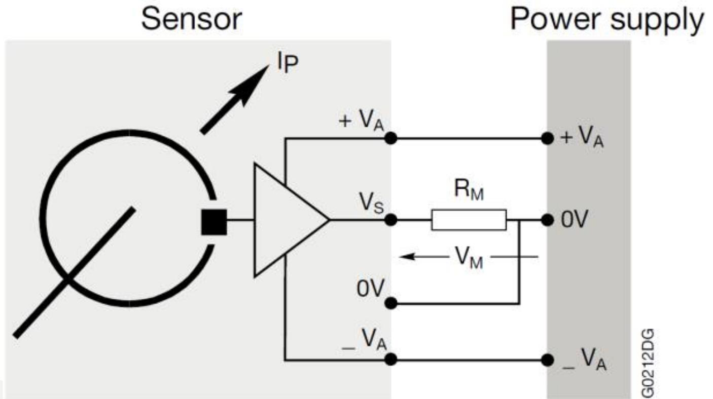
Schematic diagram: RFCS sensor (open loop technology)
