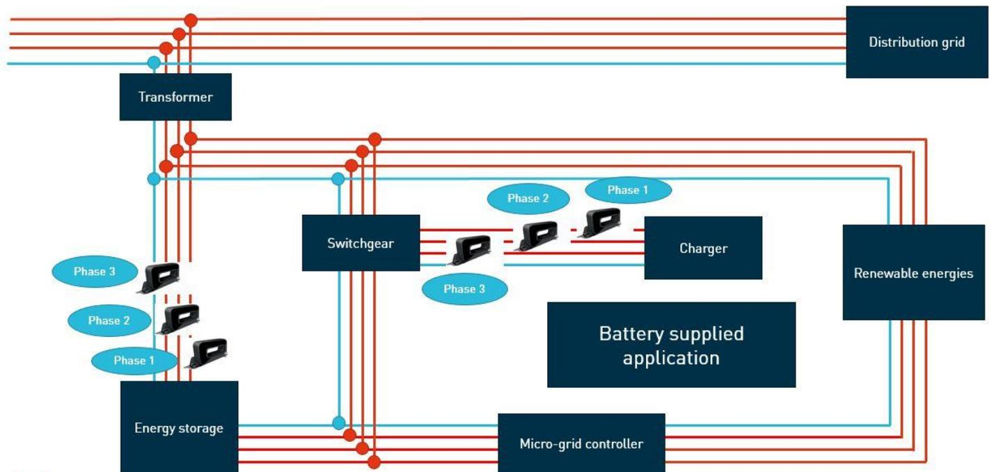
Each renewable energies (windmill, solar...) is either connected to the micro grid controller or the transformer. The energy storage is an assembly of a battery (in series and/or parallel), consequently, it can be mandatory for your application to install on each phase one RFCS sensor due to the fact you can have a variation of a significant current on the network.
