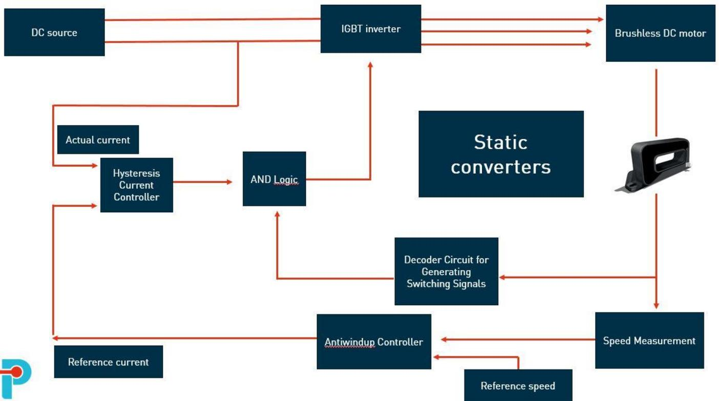
Each brushless DC motor are linked to RFCS current sensors (Hall sensor) on each phase of the motor. The RFCS will measure instantaneously on each phase the current. On the one hand, this value will serve for controlling the speed measurement as well give the value to the decoder circuit for generating switching signals.
