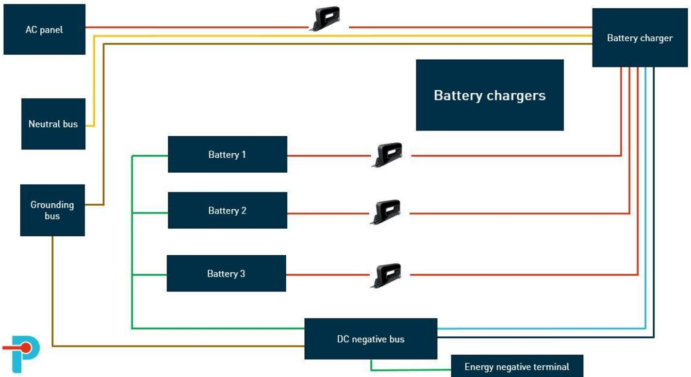
Each battery charger can be an opportunity to use our RFCS current sensors on each battery (3 RFCS in total) and upstream the battery charger linked to the AC panel (3 more RFCS sensors).. Each battery (1 phase/DC) is linked to the battery charger. Each battery is connected to DC negative bus in order to close the electrical circuit.
