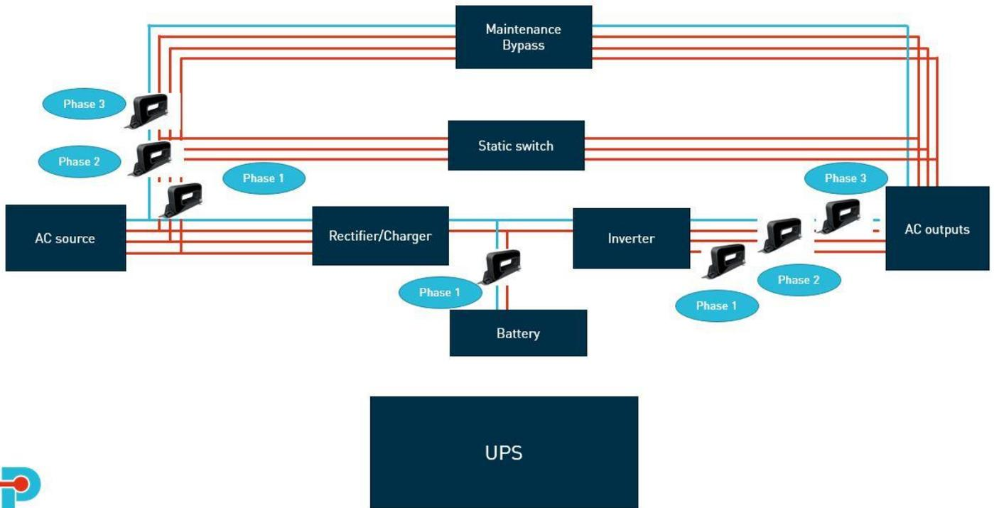
Internal design of a multi-mode UPS.
