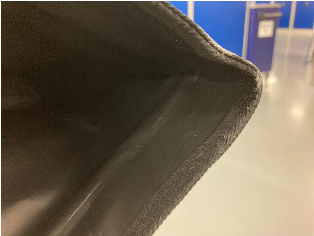
Figure 4: No dust was detected in the EUT.
