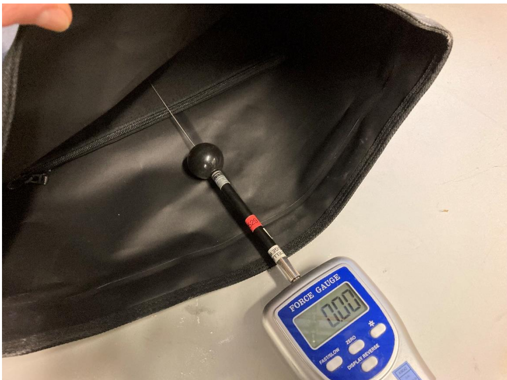
Figure 7: The 1-mm-wire probe entered the EUT.
