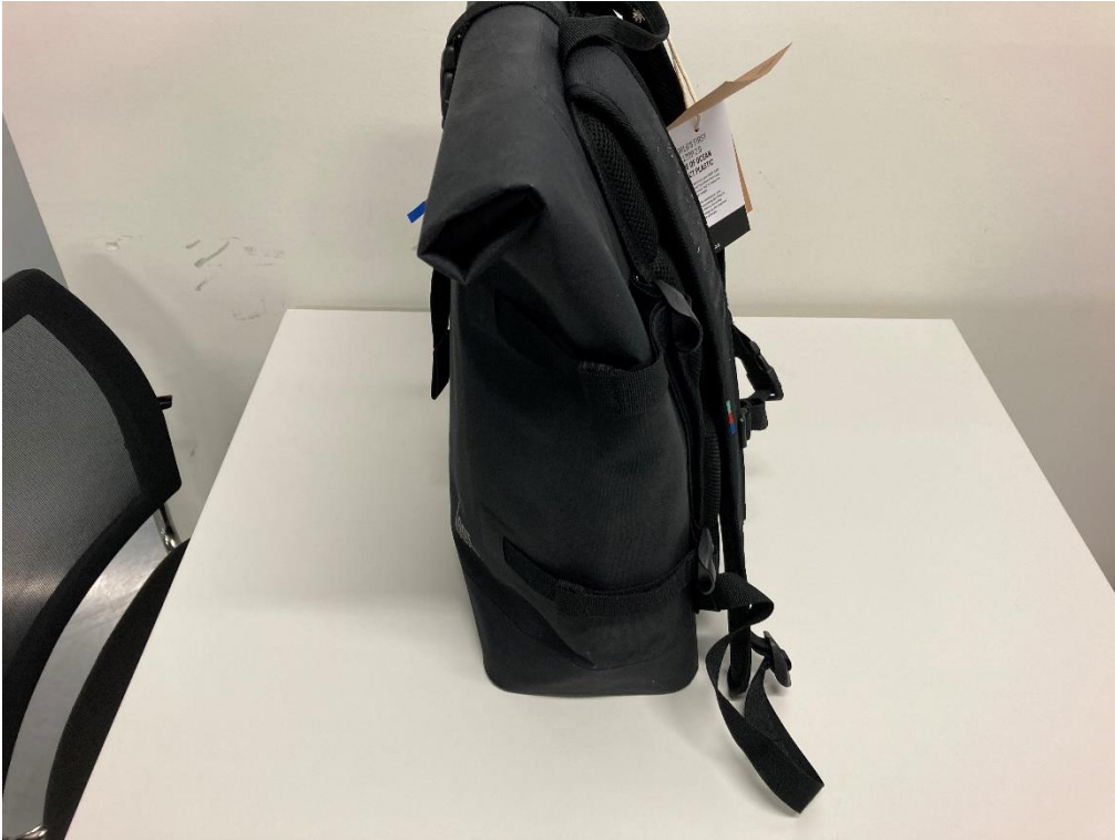
Figure 2: EUT filled with packaging material at the request of the client to perform the IPX4 test.
