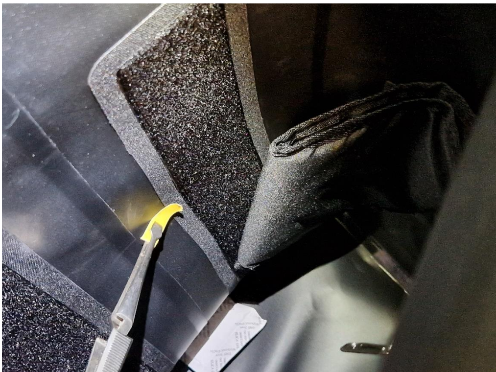
Figure 12: EUT 02 without visible ingress of water.
