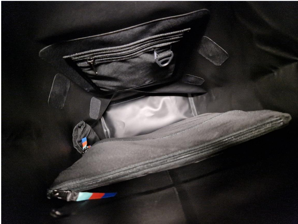
Figure 9: EUT 02 without visible ingress of water.
