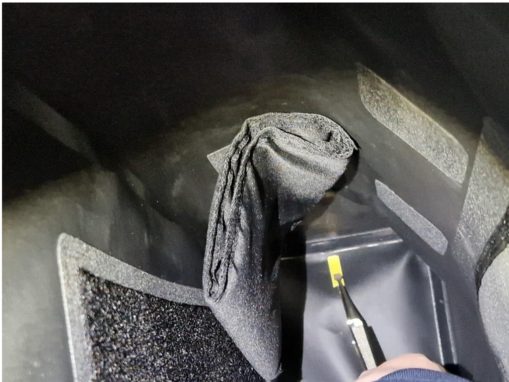
Figure 10: EUT 02 without visible ingress of water.
