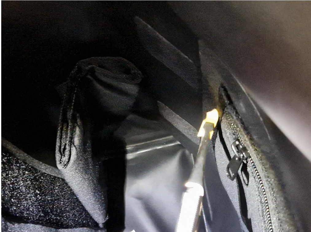
Figure 11: EUT 02 without visible ingress of water.
