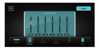
In the **Guitar Tones** menu, select a preset and click **Edit** to adjust its parameters. Nova Go Sonic has six effects: Noise Reduction, Speaker Simulation, EQ, Modulation, Delay, and Reverb. Rotate the knob to adjust: clockwise to increase, counterclockwise to decrease. For EQ, slide up to increase, down to decrease. In the effects chain, click to select and adjust effects; a highlighted module indicates selection. Slide to turn effects on/off; inactive modules appear higher and darker.
