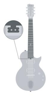
The Nova Go Sonic's neck is made of carbon fiber, offering better stability than wood. However, prolonged exposure to certain environments may still cause deformation. Considering some users' preference for personalized string action, Nova Go Sonic retains a traditional guitar truss rod for neck adjustment.
