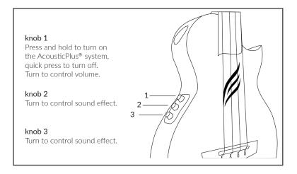
The AcousticPlus® uses as a regular acoustic-electric system as well. The output jack locates on the bottom of the ukulele body.
