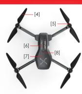
[4] Propeller Blade [5] Motor [6] Power Indicator [7] Intelligent Battery [8] Power Button
